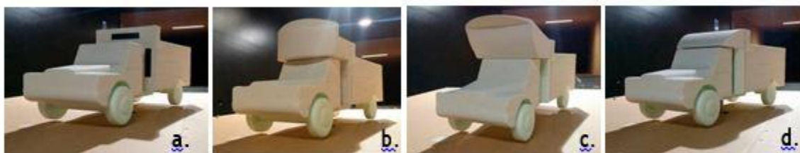
Fig. 5. Experimental setup inside the RMIT Industrial Wind Tunnel test section. Baseline truck fitted with deflector: (a) Bangladeshi, (b) Pakistani, and (c) Aerodynamic
