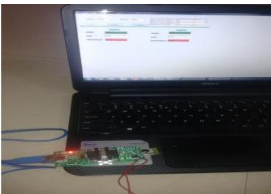
Figure5: Zigbee receiver with cloud based application
