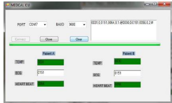
Figure7. cloud based monitoring GUI
