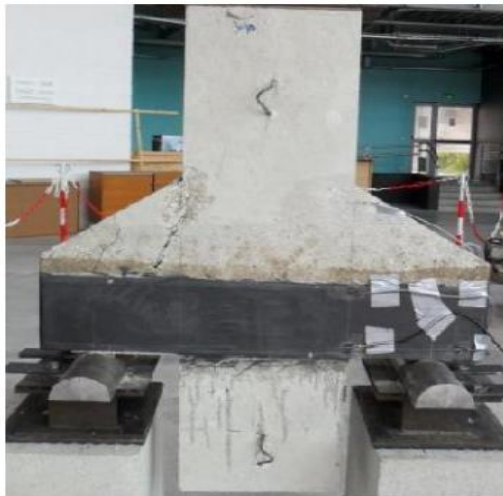
b) CB3u : Compression failure
