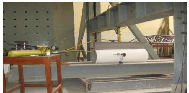
Figure 7. Pipe testing and loading system.
