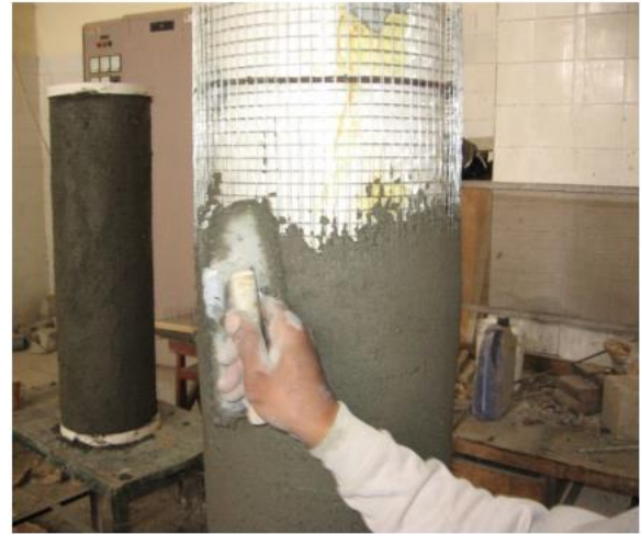
Figure 6. Casting the pipe by plastering.
