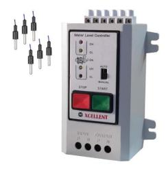
the overhead tank is full. The pump is not allowed to start if the water level in the sump tank is low This water level controller monitors the level of overhead tank and automatically switches ON the water pump whenever the level goes below a limit. The level of the overhead tank is indicated using a LED'S and the pump is switched OFF when.
