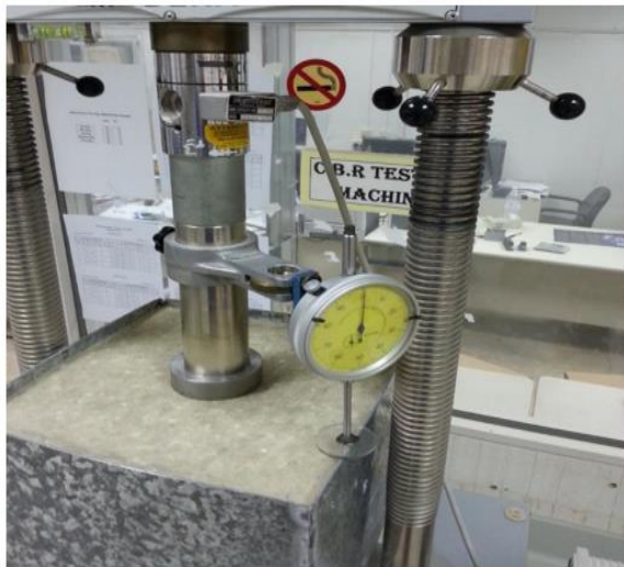
Figure 6a. Load test set up on clayey sand (catch) soil.
