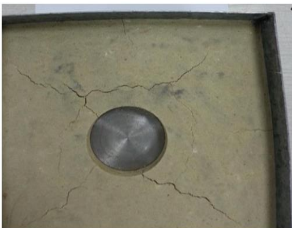
Figure 6b. After failure view showing punching failure and radial cracks (RC = 90%).
